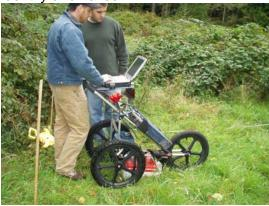
SubTerra staff laid out radar survey lines on a 5-ft by 5-ft grid then followed Structure Radar Imaging flagging and photographing anomalies as they were identified.
