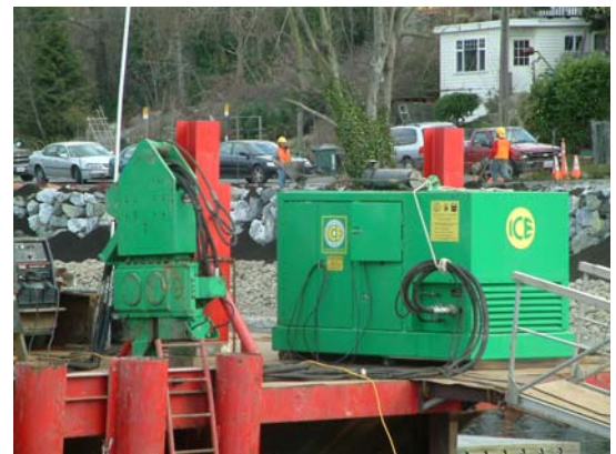
This photograph shows the ICE Vibratory Hammer and power pack located on the dock.
