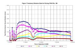
The chart above shows plotted, time phased data for Pile No. 6. These data confirm that maximum vibrations occur during initial pile driving and decrease with depth. Measured impacts were not impactive to off site structures.
